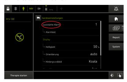
4. Select "Alarm volume 2" or higher and the corresponding alarm tone will be emitted once. Then press the confirm button. Now, you are guaranteed to have an acoustic alarm signal when the alarm goes off.
